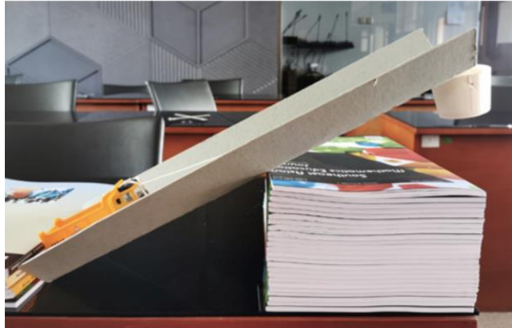
Figure 2. The gradient test with cardboard ramp.
